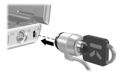
3. Turn the key counterclockwise **1**, remove the key **2**, and keep it in a safe location.
